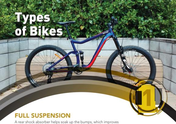
A rear shock absorber helps soak up the bumps, which improves handling and comfort. Rear suspension does add weight – and expense – to the bike, but has become an extremely popular option due to the confidence it gives and the fact that it enables you to tackle more challenging terrain.
